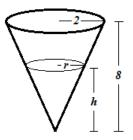
We know that  $\frac{dV}{dt} = -2$ , and we want to compute  $\frac{dh}{dt}$  when h = 4. Since we're not given any information about r, we can eliminate it from the volume formula using the usual similar triangle method ("flatten" the cone to obtain two concentric similar triangles): this yields  $\frac{2}{r} = \frac{8}{h} \Rightarrow r = \frac{h}{4}$ . Thus,
